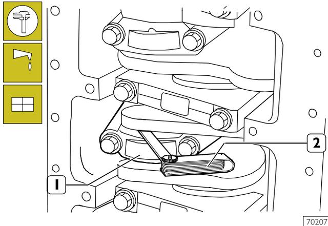
If a different clearance value is found, replace the half bearings and repeat the check.
