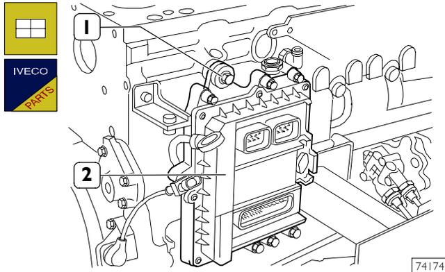
Assemble the electronic gearbox (2) equipped with the exchanger to the engine, fixing it with the screws (1). In case the rubber buffers are cracked or excessively deformed, provide replacing them.
