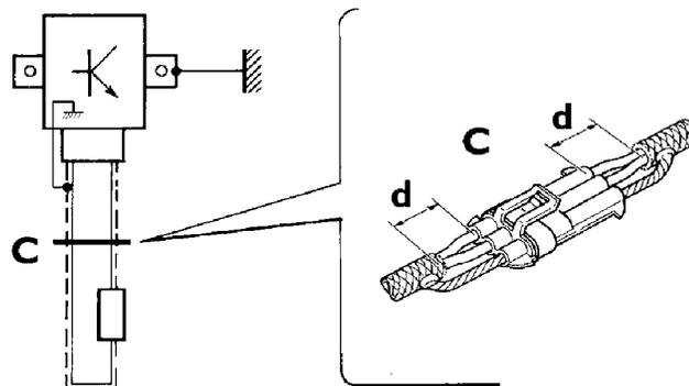
2. SCREENING THROUGH METALLIC BRAIDING OF A CABLE TO AN ELECTRONIC COMPONENT – C. CONNECTOR
