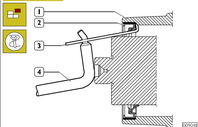
Using the specific tie rod (3) of the tool 99363204 and the ancillary lever (4), remove the external holding ring (2) from the front cover (1).
