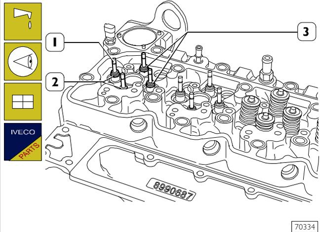
Lubricate the valve stems (1) and fit them into the relevant valve guides according to the position marked at removal. Fit the sealing rings (2 and 3) on the valve guide.
