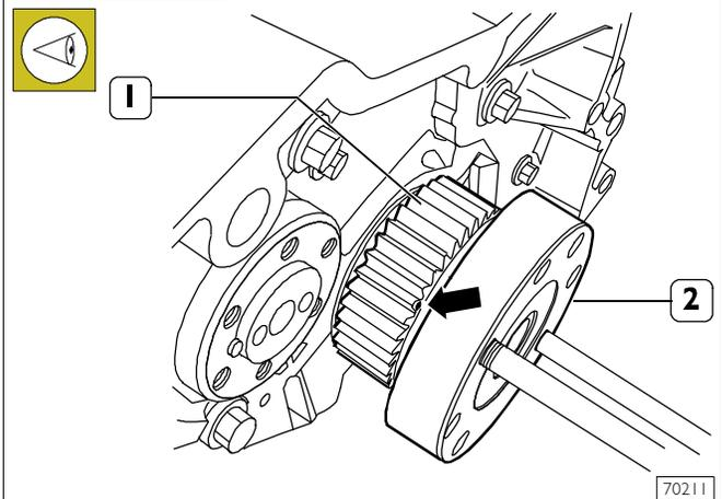
Use a felt pen to mark the driving gear (1) tooth fitted on the output shaft (2) having the mark (→) for timing on the side surface.
