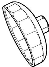
Tool to remove oil filter (engine)
