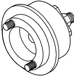
Tool for fitting output shaft rear gasket
