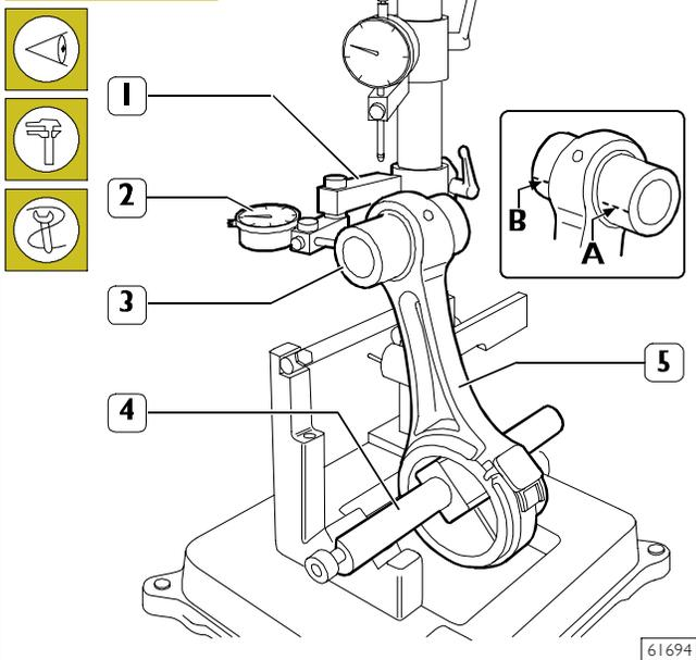
Check connecting rod (5) torsion by comparing two points (A and B) of pin (3) on the horizontal plane of the connecting rod axis.
