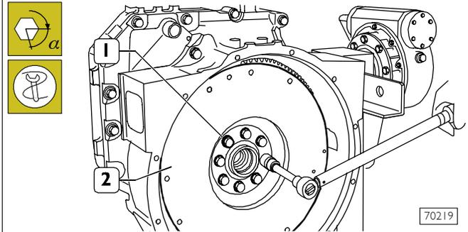
Tighten engine flywheel (2) fastening screws (1) in two stages:
