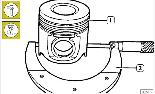
Using a micrometer (2), measure the diameter of the piston (1) to determine the assembly clearance.
