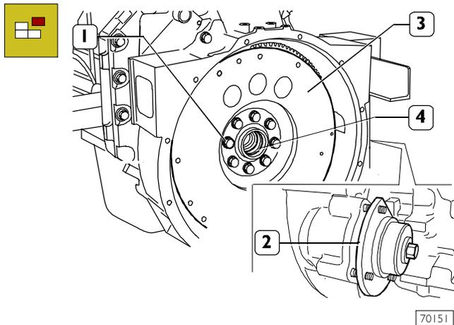
Remove two opposite screws (1) from the area where the withdrawal pins will be introduced (2, Figure 29). Loosen the remaining flywheel fixing screws (3) from the driving shaft (4). Remove the flywheel locking tool 99360351.
