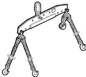
Lifting rig for engine removal/refitting
