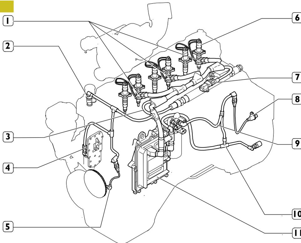
1. Connections for Electro-injectors - 2. Engine cooling liquid temperature's sensor - 3. Cable of the fuel pressure sensor - 4. Sensor of engine's oil temperature and pressure - 5. Driving shaft sensor - 6. Electro-injector - 7. Temperature - air pressure sensor - 8. Timing system sensor - 9. Cable of fuel heater and fuel temperature's sensor - 10. Cable of pressure regulating gauge - 11. EDC 7 gearbox.
