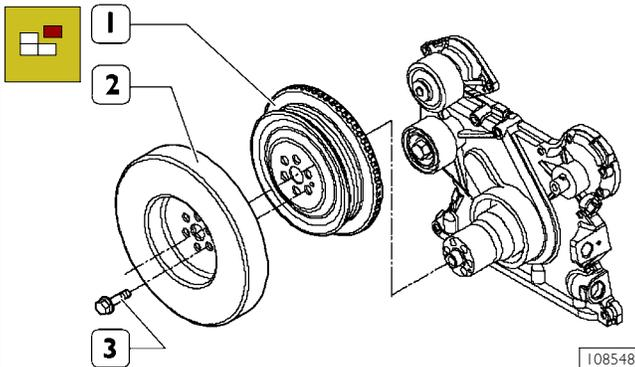
Remove the screws (3) and disassemble the damping flywheel (2) and the pulley (1).
