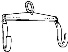
Tool for lifting the output shaft
