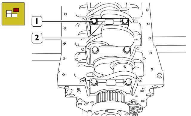
Remove the screws (1) and the main bearing caps (2).
