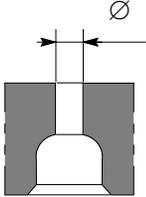
Valve guide seats on cylinder head                                | $\varnothing 1$                                                                                                                                                                                                                    | 7.042 to 7.062                                                                 |
