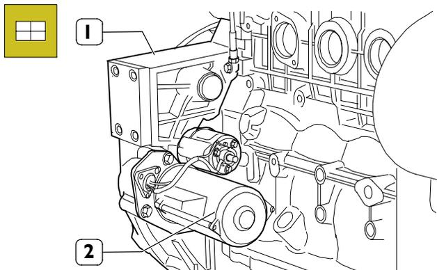
Assemble the starter (2) to the internal part of the flywheel cover.
