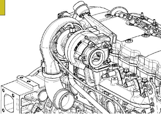
Remove the screws and remove the oil pipe (1) from the turbocharger pipe (2) and from the engine block.
