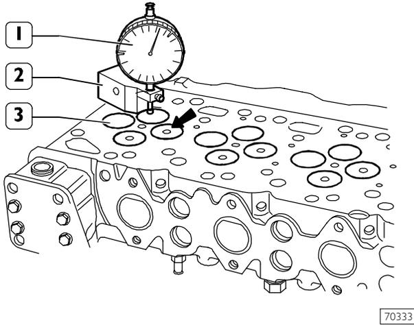
After regrinding, check that valve (3) sinking value is the specified one by using the base 99370415 (2) and the dial gauge 99395603 (1).
