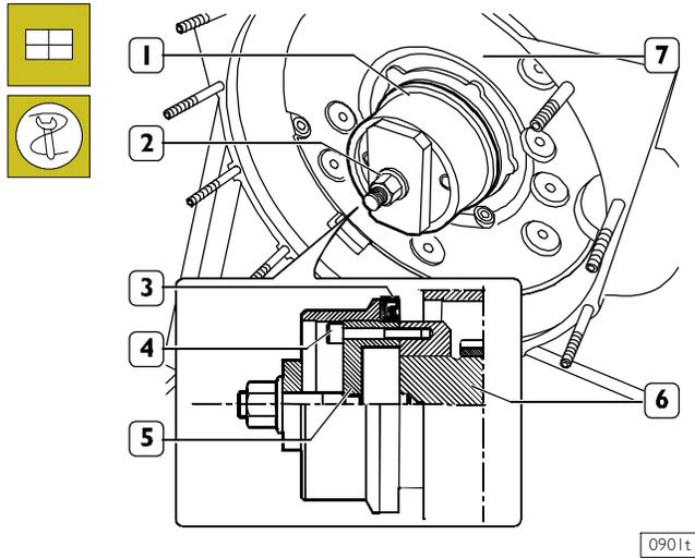
Apply tool 99346252 part (6) to the rear output shaft tang (5), secure it by screws (4) and fit the new sealing ring (3). Position part (1) on part (5), screw nut (2) until completing sealing ring (3) fitting into flywheel housing (7).
