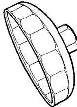
Tool to remove oil filter (engine)
