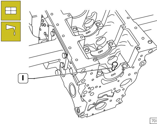
Lubricate the tappets (1) and fit them into the relevant housings on the engine block.
