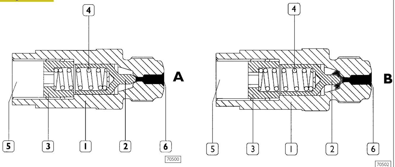
1. Body – 2. Small piston – 3. Stop – 4. Spring – 5. Direct tank discharge – 6. Seat on rail.
