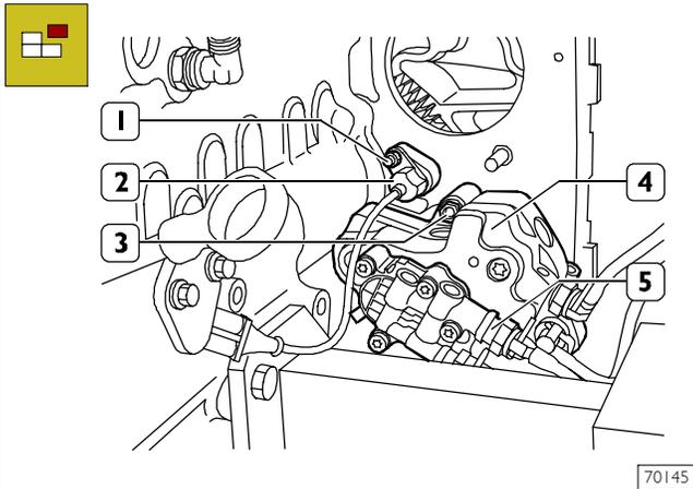
Remove the nut (1) and disconnect the timing sensor (2).
