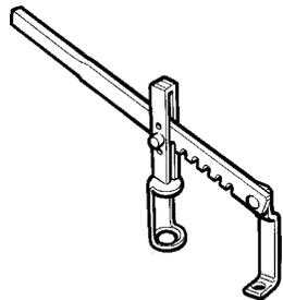
Tool for removing/refitting engine valves
