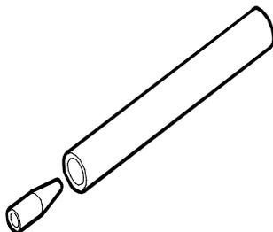
Keying device for seal assembly on the valve guide
