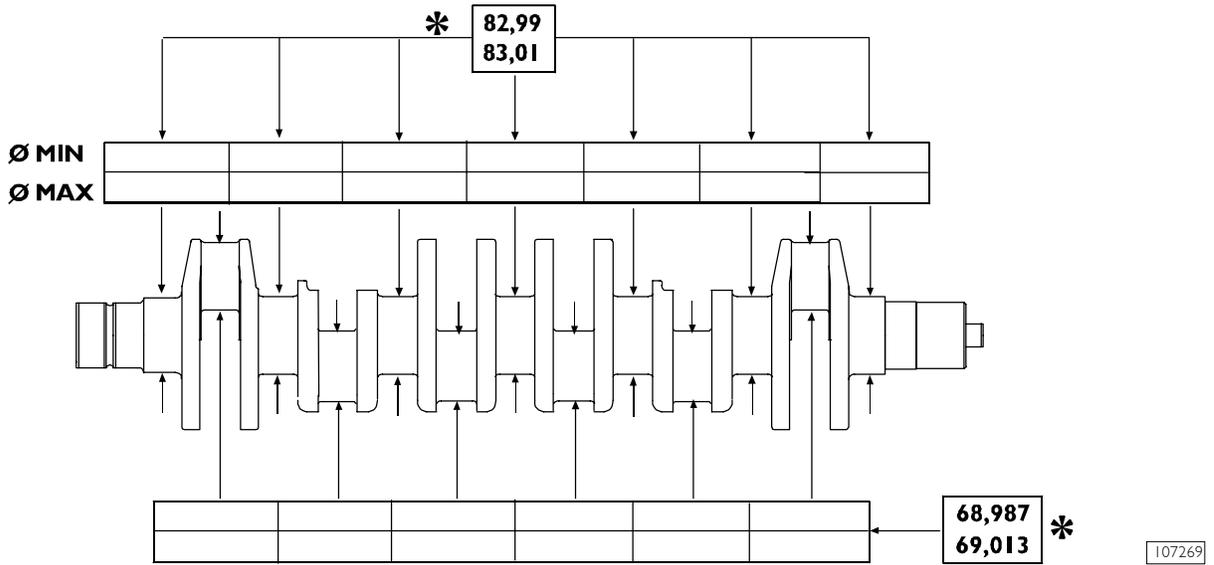
FILL THIS TABLE WITH OUTPUT SHAFT JOURNAL AND CRANKPIN MEASURED VALUES
