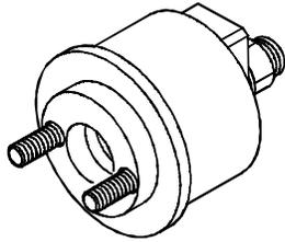
Tool for fitting output shaft front gasket
