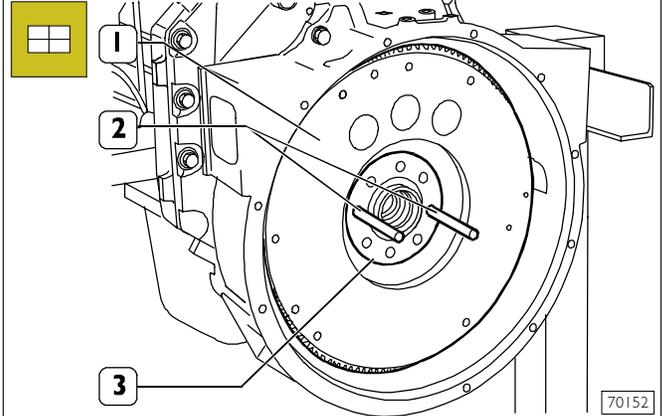
Screw two pins (2) having suitable length into shaft holes (3) and remove the engine flywheel (1) using proper sling and hoister.
