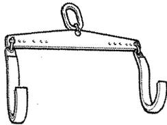
Tool for lifting the output shaft
