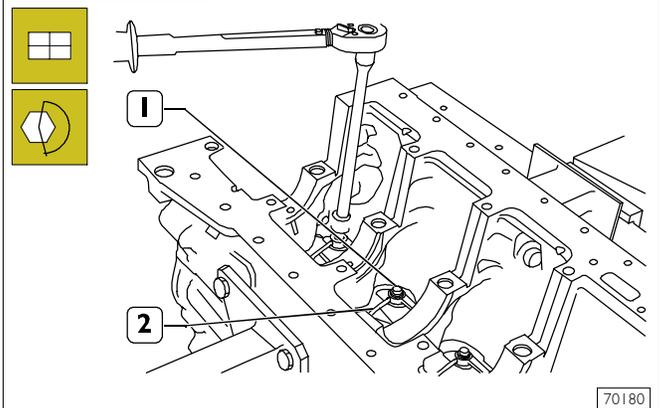
Fit nozzles (2) and tighten the fastening screws (1) to the specified torque.
