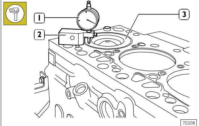
Once connecting rod-piston assemblies refitting is over, use dial gauge 39395603 (1) fitted with base 99370415 (2) to check piston (3) protrusion at T.D.C. with respect to the top of the engine block.
