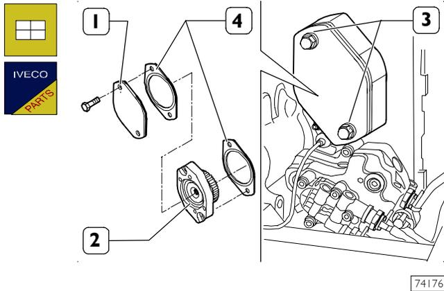
Insert the power take-off (2) equipped with the gasket (4), the cover (1) and its gasket (4). Tighten the screws (3) to the prescribed matching couple.
