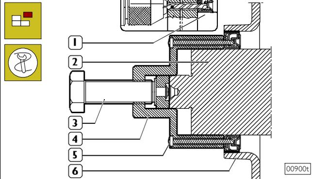
Remove the ring sealing the engine's driving shaft from the front cover. Use the tool 99340055 (4) to operate on the front bar hold of the driving shaft. Through the steering holes of the tool, perforate the inside holding ring (1) with a straight way drill (diam. 3,5mm) for the depth of 5mm. Fix the tool to the ring tightening the 6 screws provided with the equipment. Then proceed removing the ring (2) by tightening the screw (3).
