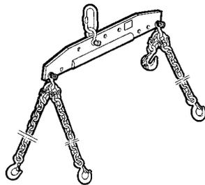
Lifting rig for engine removal/refitting
