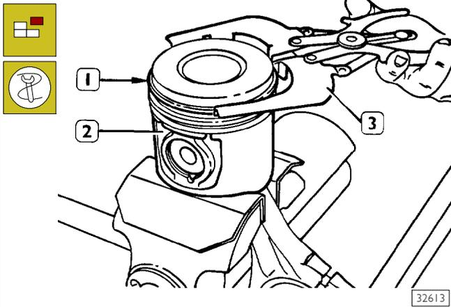
Remove split rings (1) from piston (2) using pliers 99360183 (3).
