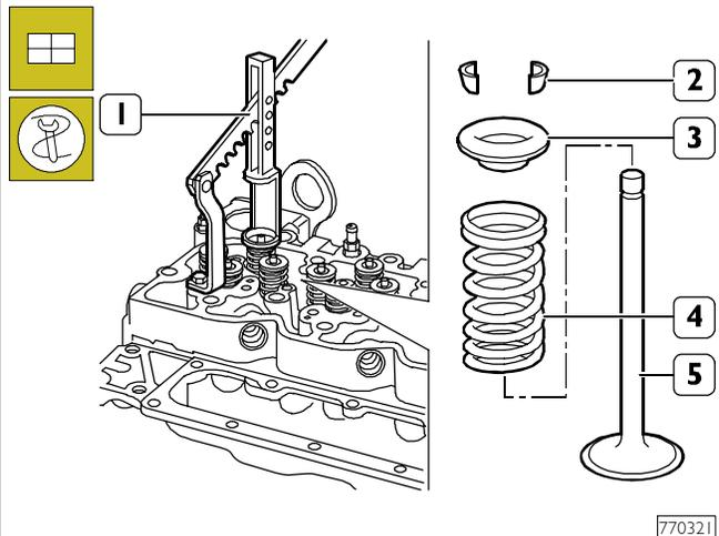
Position on the cylinder head: the spring (4), the upper cap (3); use tool 99360268 (1) to compress the spring (4) and lock the parts to the valve (5) by the cotters (2).
