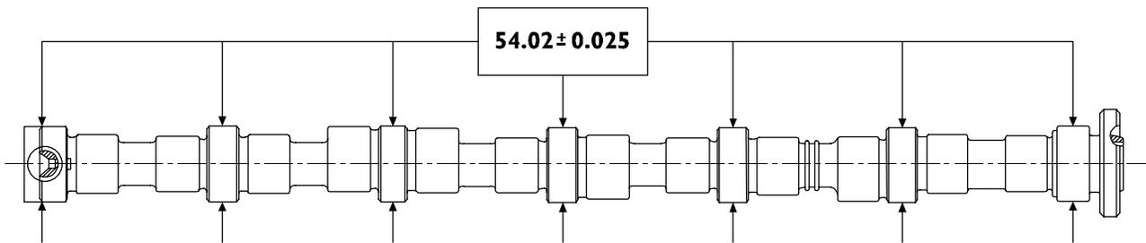
MAIN DATA ABOUT CAMSHAFT PINS (6 F4HE684 engine cylinders)
