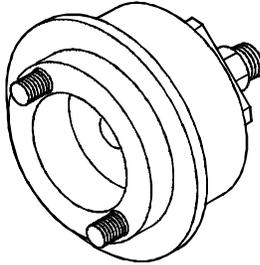
Tool for fitting output shaft rear gasket
