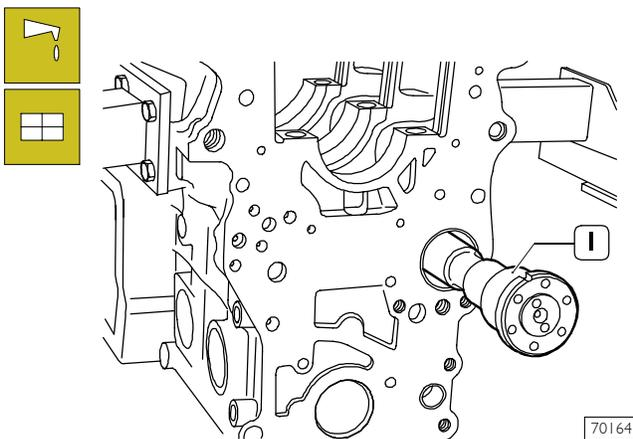
Lubricate the camshaft bushes and fit the camshaft (1) taking care not to damage the bushes or the housings.
