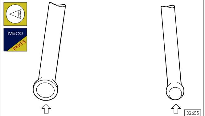
Rocker control rods shall not be distorted; the ball seats in touch with the rocker adjusting screw and with tappets (arrows) shall not show seizing or wear; otherwise replace them. Intake and exhaust valve control rods are identical and are therefore interchangeable.
