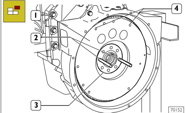
Tighten two screws of medium length into the holes (4) to sling the flywheel with the hoist.
