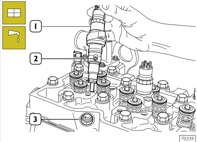
Fit injectors (1) on the cylinder head seats, directed so that the fuel inlet hole (2) is facing the fuel manifold seat (3) side.
