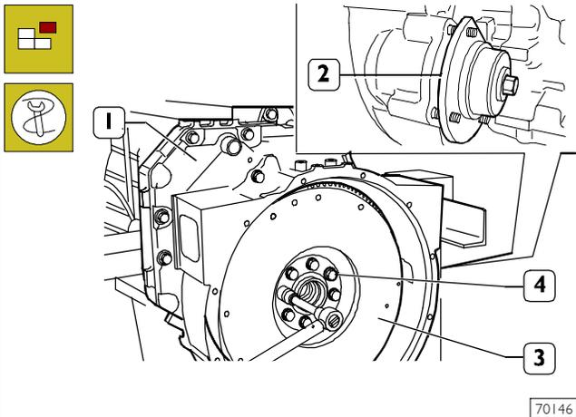
Fit tool 99360339 (2) to the flywheel housing (1) to stop flywheel (3) rotation.
