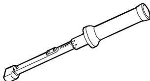
Dog type dynamometric wrench 9x12 (5-60 Nm)
