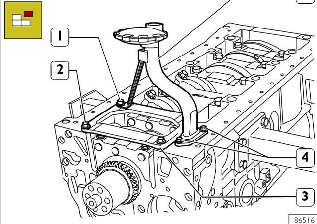
Remove the screws (1 and 4) and disassemble the oil suction tube (5). Remove the screws (2) and disassemble the stiffening plate (3).
