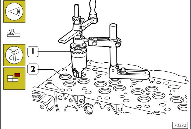
Check the valve seats (2). If slight scoring or burnout is found, regrind seats using tool 99305018 (1) according to the angle values shown in Figure 81.
