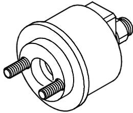
Tool for fitting output shaft front gasket
