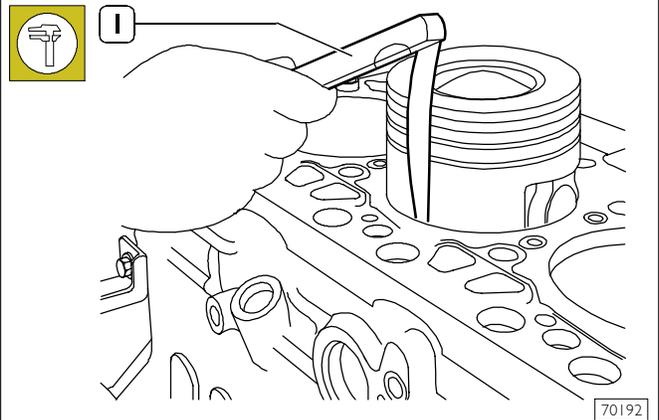
The clearance between the piston and the cylinder barrel can be checked also with a feeler gauge (1) as shown in the figure.
