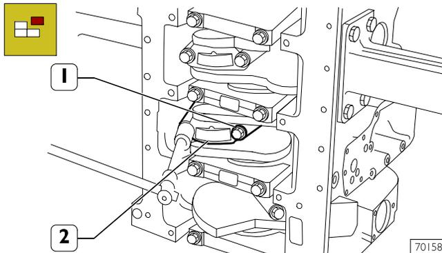
Loosen the fixing screws (1) and remove the rod caps (2).
