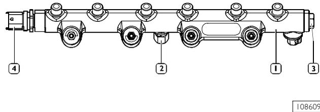
1. Rail – 2. Fuel inlet from high-pressure pump –
