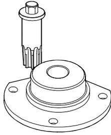
Tool for rotating/stopping the engine flywheel
