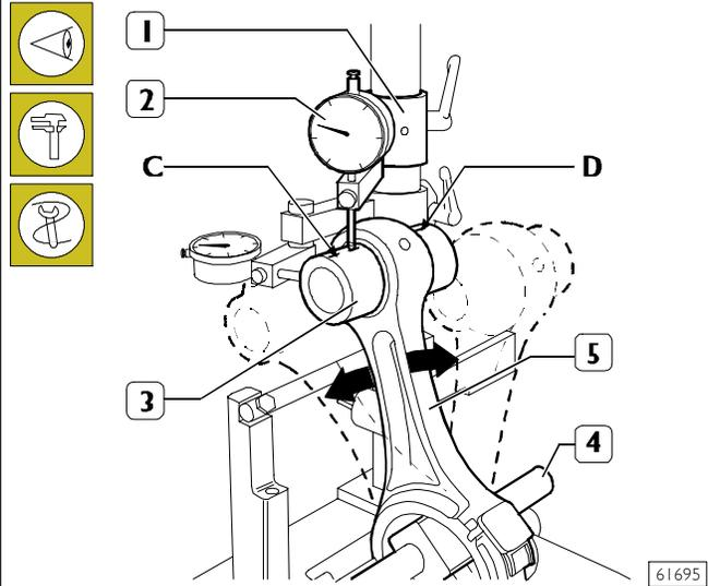
Check connecting rod (5) bending by comparing two points C and D of the pin (3) on the vertical plane of the connecting rod axis.
