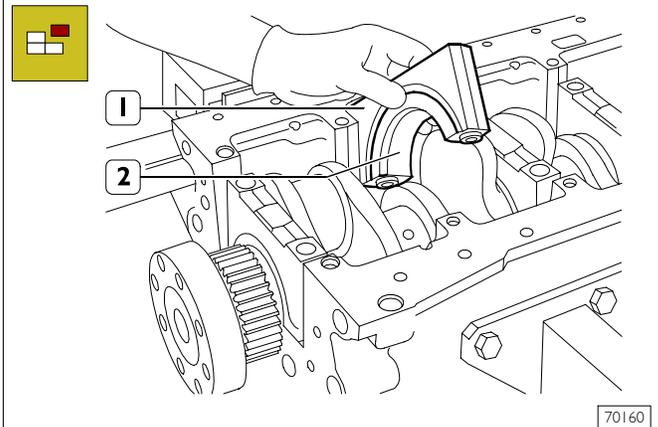
The second last main bearing cap (1) and the relevant support are fitted with shoulder half-bearing (2).
