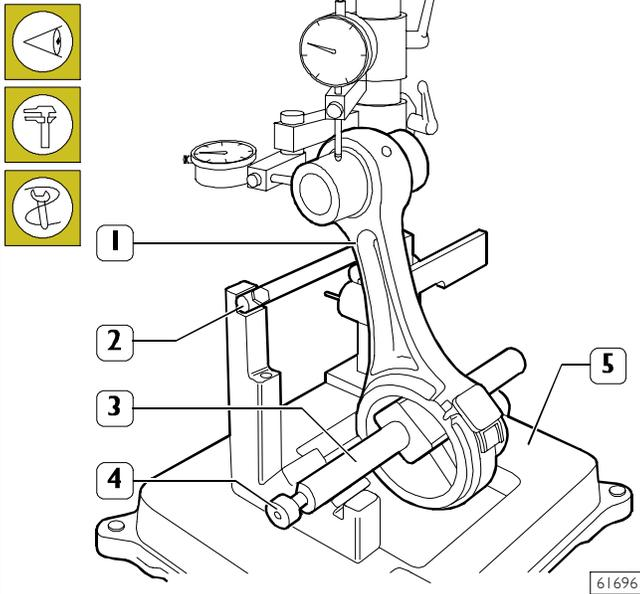
Check that the axis of the connecting rods (1) are parallel using tool 99395363 (5) as follows:
