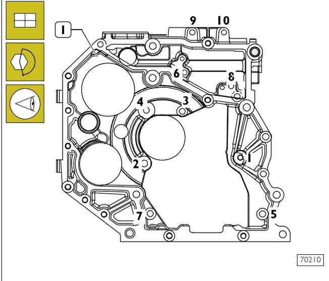
**DIAGRAM FOR TIGHTENING THE REAR TIMING GEAR CASE FASTENING SCREWS**
