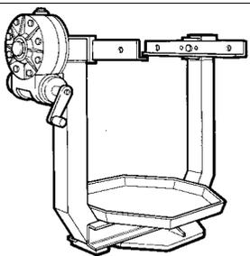
Revolving stand for overhauling units (700 daN/m capacity, 120 daN/m torque) |
