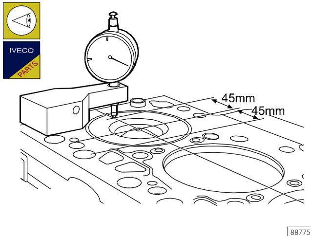
There are two types of head seals for F4AE04., F4AE06. and F4HE06. engines, for the thickness (1.25 mm Type A and 1.15 mm Type B) take the following measures:
