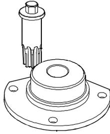
Tool for rotating/stopping the engine flywheel
