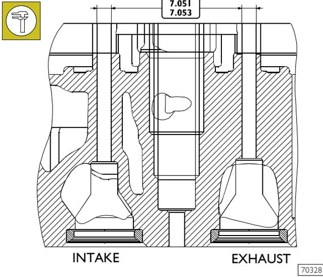
Use a bore dial gauge to measure the inside diameter of the valve guides, the read value shall comply with the value shown in the figure.
