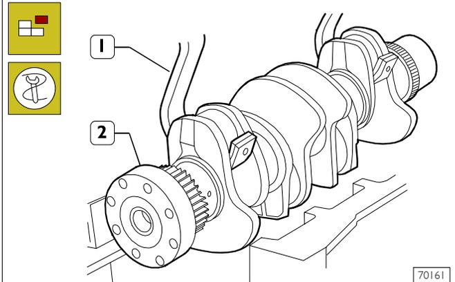
Use tool 99360500 (1) and hoist to remove the crankshaft (2) from the block.
