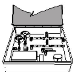
Tool to check the diesel supply circuit and the common-rail injection system  |
