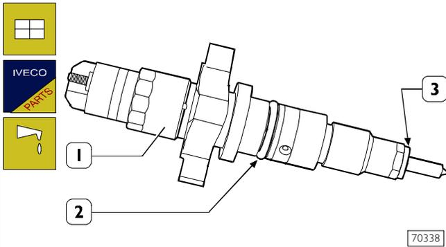
Fit a new sealing ring (2) lubricated with petroleum jelly and a new sealing washer (3) on injector (1).
