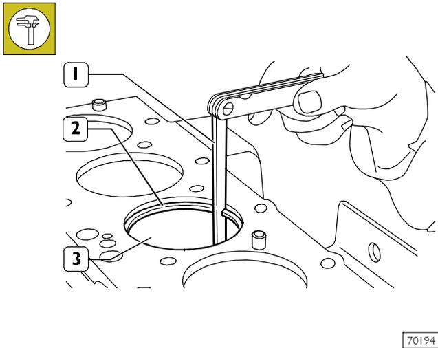
Use feeler gauge (1) to measure the clearance between the ends of the split rings (2) fitted into the cylinder barrel (3).
