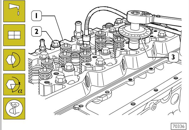
Assemble cylinder head (1), tighten the screws (2) in three following steps, following order and mode shown in the figure below.
