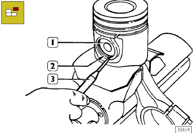
Piston pin (1) split rings (2) are removed using a scriber (3).
