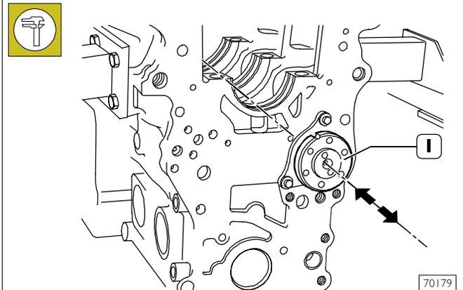
Check camshaft end float (1). It shall be  $0.23 \pm 0.13$  mm.
