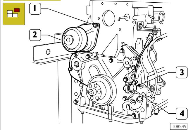
Remove the screws (1) and disconnect the water pump (2).
