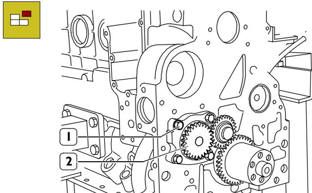
Remove the screws (1) and disconnect the oil pump (2).
