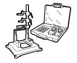
Complete square to check for connecting rod distortion
