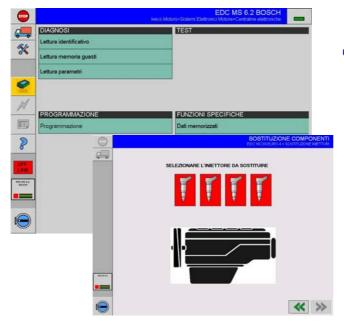
The specific functions allow, in case of ECU, engine or injector replacement, to update the ECU to the new configuration in one of the three replacement cases mentioned above.
