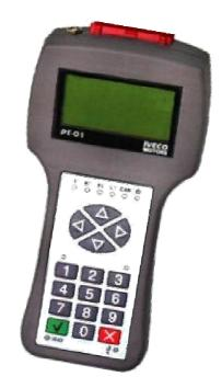
With the PT-01 portable tester, it is possible to diagnose and inquire the ECUs controlling the IVECO MOTORS engine injection. The PT-01 portable tester has been designed for use on the field, in the workshop and in the industrial environments.
