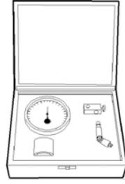
A rectangular box containing a dial gauge and other accessories.                                            | All-purpose goniometer/Inclinometer                                    |
