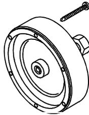
Tool to remove output shaft rear gasket
