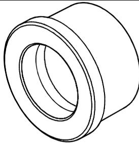
Beater for removing/refitting camshaft bushes (to be used with 993700069)
