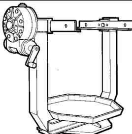
A heavy-duty metal stand with a rotating top section and a base.                                       | Revolving stand for overhauling units (700 daN/m capacity, 120 daN/m torque) |
