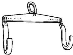
Tool for lifting the output shaft
