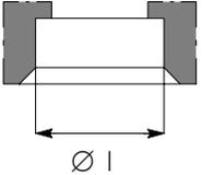
Housing on head for valve seat:                                 | Ø 1<br>Ø 1                            | 34.837 to 34.863<br>34.837 to 34.863                           |
