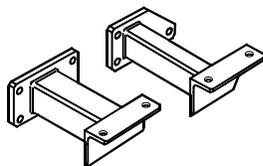
Brackets for fastening engine to revolving stand 99322205
