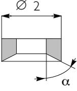
Valve seat outside diameter; valve seat angle on cylinder head: | Ø 2<br>α<br>Ø 2<br>α                  | 34.917 to 34.931<br>60°<br>34.917 to 34.931<br>45°             |
