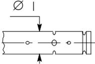
Rocker shaft <span style="float: right;">Ø 1</span>                         | 21.965 to 21.977                      |                                       |
