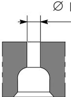
Valve guide seats on cylinder head                                | Ø 1                                   | 7.042 to 7.062<br>7.042 to 7.062                               |
