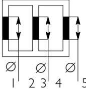
Camshaft bush housings No. 1-5/1-7<br>Camshaft housings No. 2-3-4/2-3-4-5-6                         |                                       | 59.222 to 59.248<br><br>54.089 to 54.139 |
