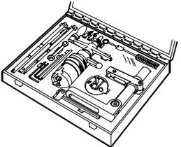
A collection of various tools including grinding wheels, guides, and brushes, organized in a metal tray. | Kit for valve seat regrinding                                                |
