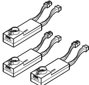
Three electronic adapters with cables and connectors.                                                  | Adapter for measures on engine injectors (use with 99395872)                 |
