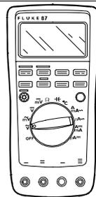
Analog to digital multimeter for voltage, current intensity, resistance, diodes, frequencies, capacity and registration of the minimum, average and maximum values
