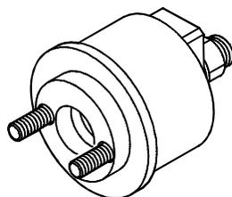
Tool for fitting output shaft front gasket
