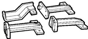
Brackets fixing the engine to rotary stand 99322230
