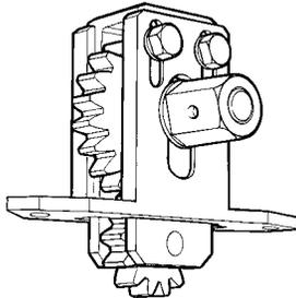
Tool to rotate engine flywheel
