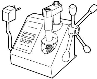
Equipment for spring load check
