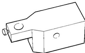
Tool to detect cylinder liner projections
