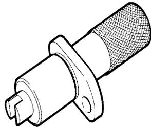
Tool for timing of phonic wheel on timing gear
