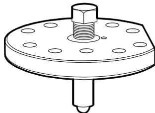
Tool for checking cylinder barrel projection.
