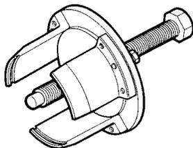
Extractor for crankshaft front gasket
