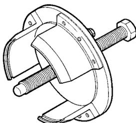
Extractor for crankshaft rear gasket
