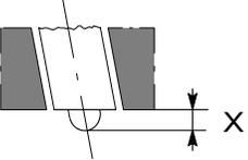
Injector protrusion X                                                                               |                       | 0.7                          |
