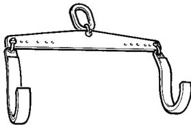
Tool to lift crankshaft
