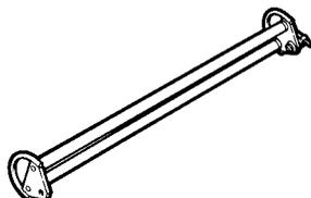
Tool to lift and transport rocker shaft
