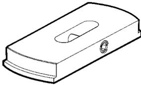
Tool to extract the cylinder liners (to be used with 99360723)
