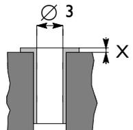
Cylinder sleeve<br>inside diameter $\varnothing 3$<br>inside diameter $\varnothing 3$<br>Protrusion                                                 | A*<br>B*<br>X          | 115.000 to 115.012<br>115.010 to 115.022<br>0.035 to 0.065                               |
