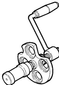
Tool to take down-fit engine valves
