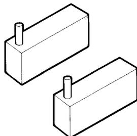
Punches (**A\*** - **B•** - **E■** - **F▲**) for printing engine identification plates (to be used with 99378100)
