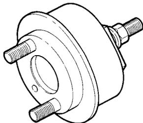
Tool to install the crankshaft rear gasket
