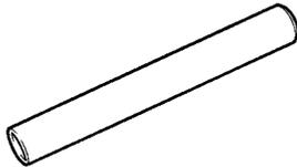
Tool to install gasket on valve guide
