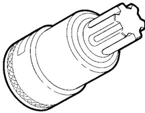
Box wrench for block junction bolts to the underblock
