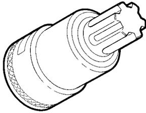
Box wrench for transmission gear support fixing screws
