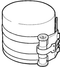
Belt to insert piston in cylinder liner (60 - 125 mm)
