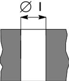
Cylinder sleeve bore<br>upper<br>lower                                                                                                               | $\varnothing 1$        | 130.200 to 130.225<br>128.510 to 128.535                                                 |
