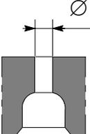
Valve guide housings in cylinder head                                      | $\varnothing 1$                                            | 12.980 to 12.997                                                                       |
