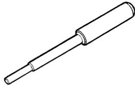
Tool to remove valve guide
