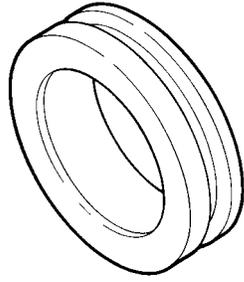
Centering ring of crankshaft front cap
