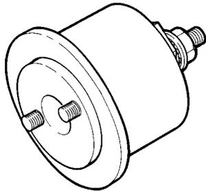
Tool to install the crankshaft front gasket
