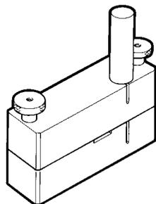
Tool for printing engine identification plates (to be used with special punches)
