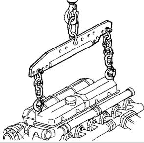
Balance for lifting and handling engine
