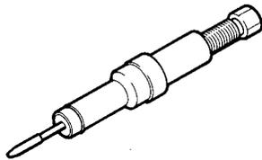
Tool for injector holder heading
