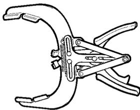
Pincers for removing and refitting circlips and pistons (105-160 mm)
