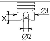
Pistons:<br>measuring dimension<br>outside diameter $\varnothing 1$ A•<br>outside diameter $\varnothing 1$ B••<br>outside diameter $\varnothing 2$ | X<br>X<br>•<br>••<br>X | 18<br>114.888 to 114.900<br>114.898 to 114.910<br>46.010 to 46.018<br>114.898 to 114.910 |
