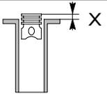
Pistons protrusion                                                                                                                                 | X                      | -                                                                                        |
